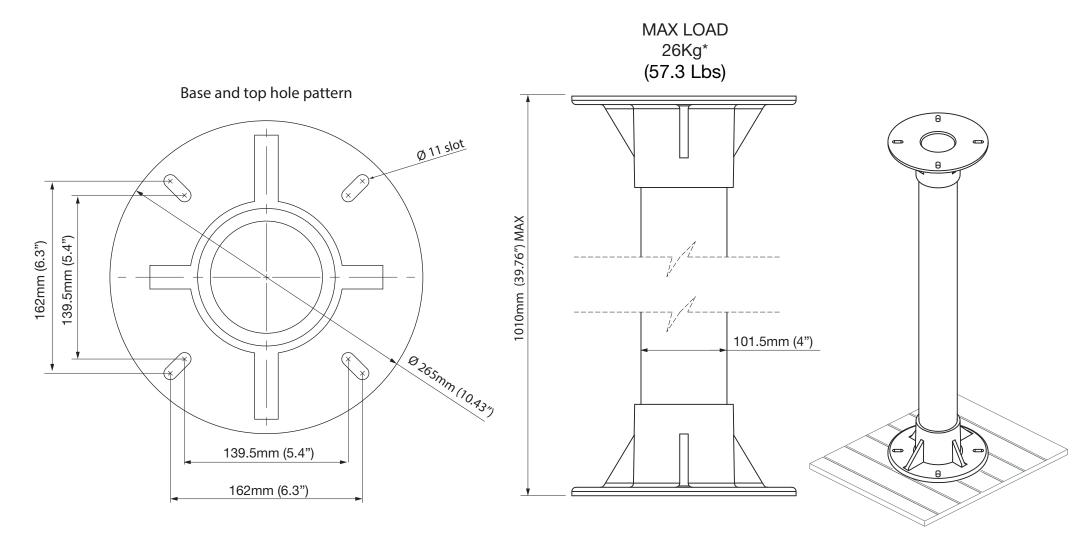
\*assuming product is installed in a dynamic environment where accelerations of up to 3g will be experienced
