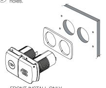
FRONT INSTALL ONLY Drill 4 pilot holes for bezel.
