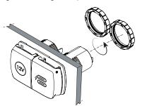
FRONT INSTALL ONLY Apply silicone seal on fixings and pilot holes.
