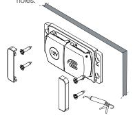
Use drilling template to drill x2 Ø32mm (1 1/4") holes (see tools required).
