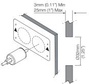
FRONT INSTALL ONLY Push bezel onto the product, make sure the bezel orientation is correct.
