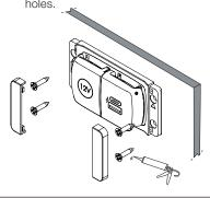
Connect to 12V supply, ensuring a waterproof connection. Fuse and select cable diameter according to input voltage and current for your specific installation.
