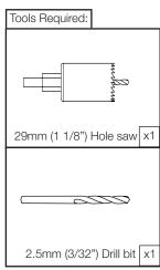
Use drilling template to drill 1 x 2.5mm (3/32") to a depth between 1-2mm, do not go through the mounting surface (see tools required).
